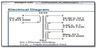
Fig 3. Electrical diagram for 16V and 5V
