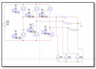
Fig 4. Three phase inverter circuit diagram
