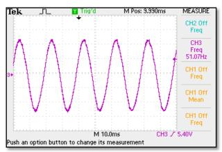
Fig 9. line voltage waveform
