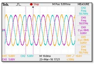
Fig 8. Three phase waveform
